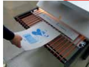
Imaged plates are fed through the integrated Finishing Unit, located below the Print Engine. This finishes the plates by drying and bonding the liquid dots to the plate surface. The Finishing Unit includes a built-in gumming station to apply a protective gum layer.
