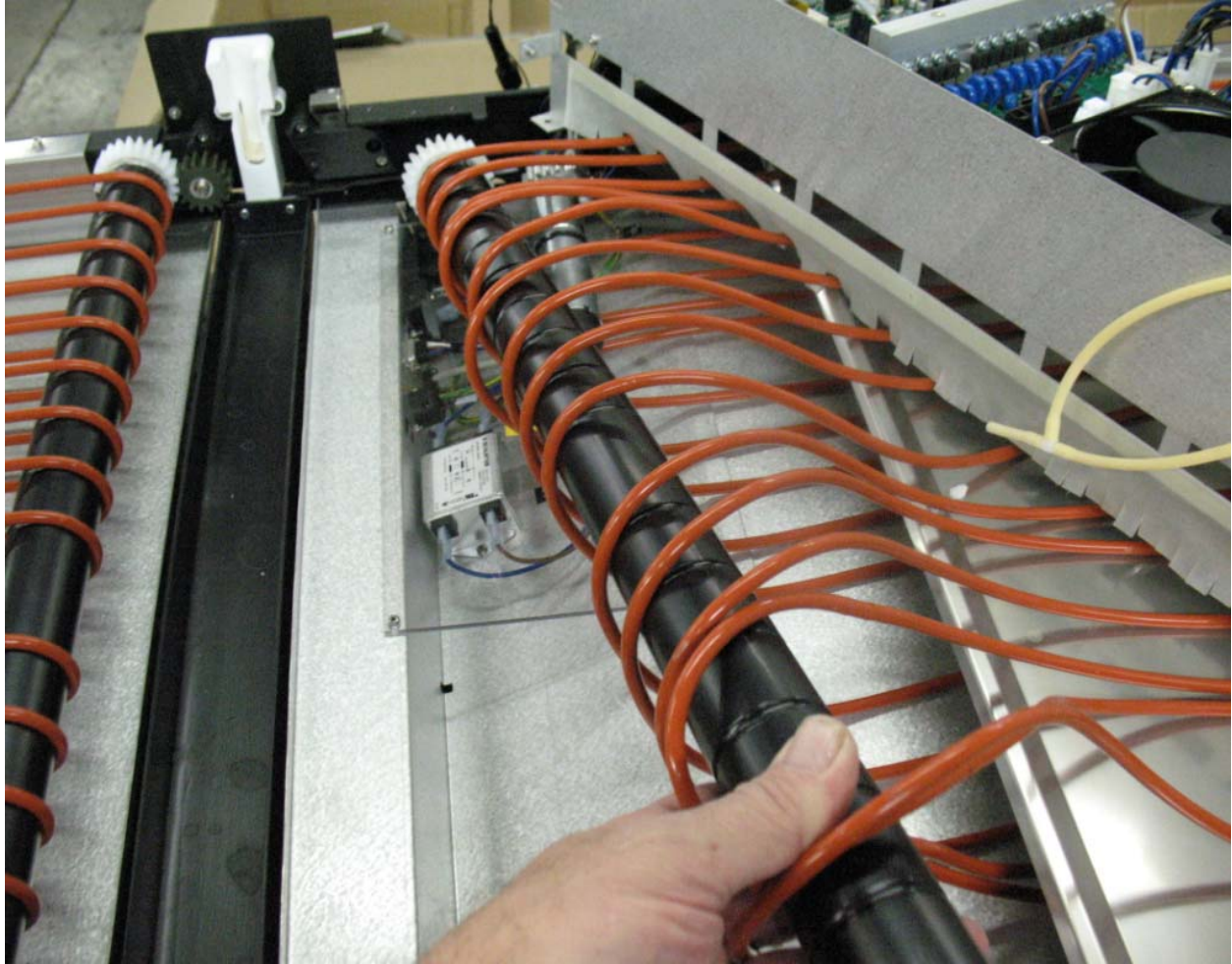
Now slide the roller out, and replace.
