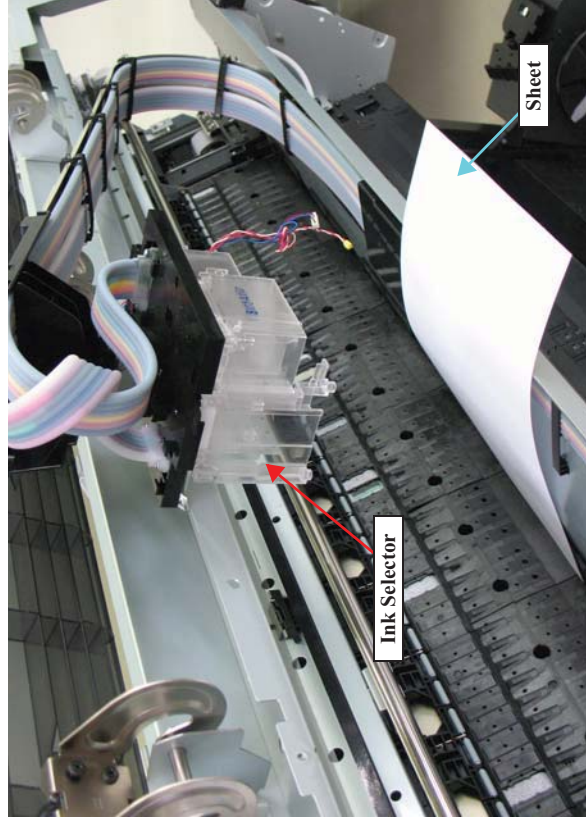
Figure 4-121. Securing the Ink Selector to the main body (2)
