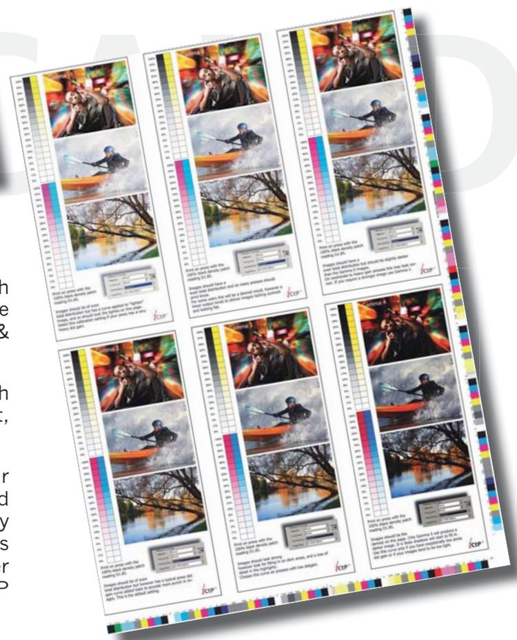
Each press sheet contains the 6 targets, each imaged with one of the 6 pre-built halftone compensations curves (programmed at Glunz & Jensen by development engineers).
